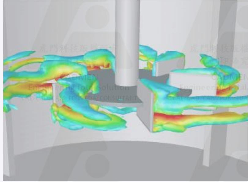
LES turbulence model predicts the occurrence of vortices behind the blade.
