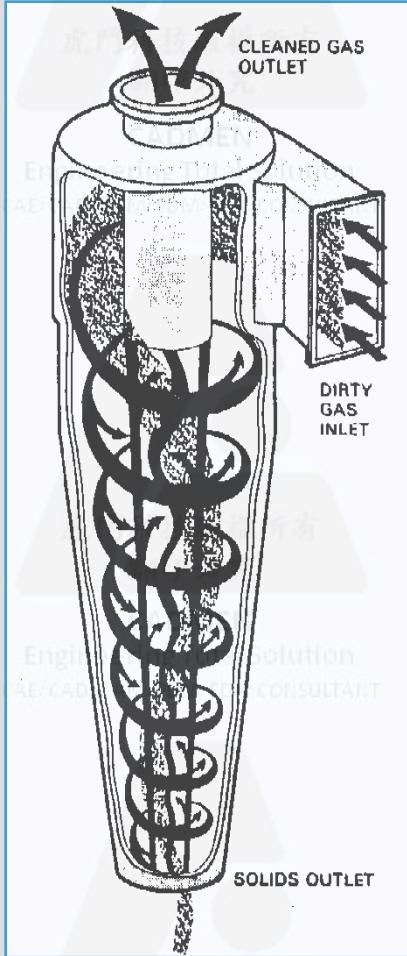
Schematic of complex flow motion in a cyclone separator
